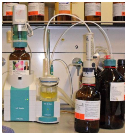
Figure 1. Volumetric reaction chamber setup (Felgner et al. , 2008), and Classical Karl Fischer titration device
