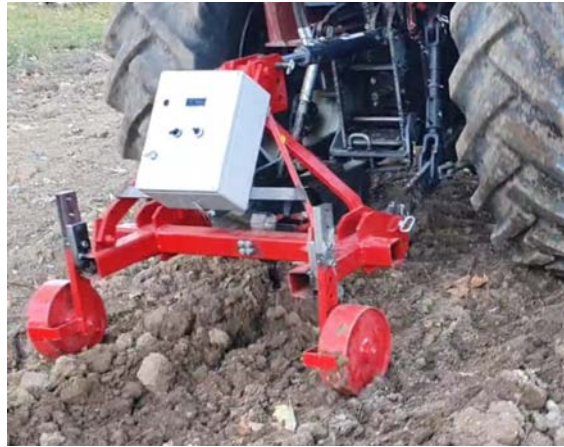
(a) (b) Fig. 8. (a) Cultivator leg-octagonal ring-three point hitch assembly, (b) The assembly mounted to the tractor in the field
